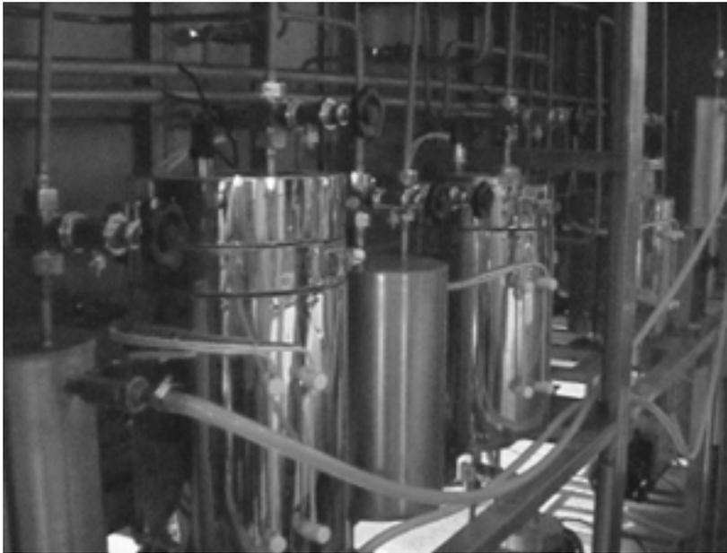
Experimental system for hydrogen isotope extraction from solid breeders
