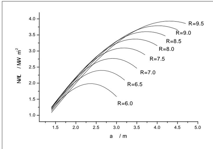
The neutron wall loading of a reactor with different sizes
