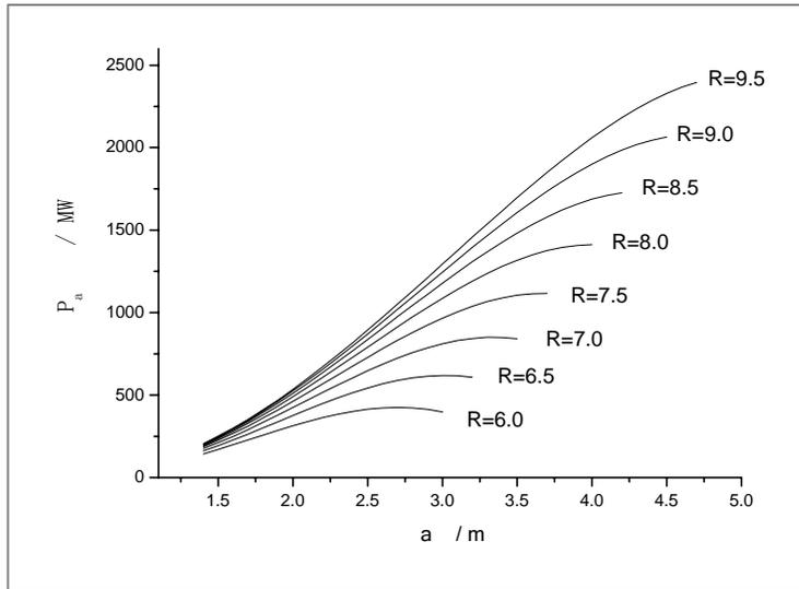
The fusion alpha power of a reactor with different sizes
