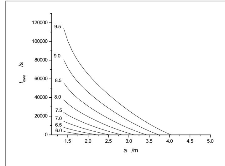
The burning time of a reactor with different sizes
