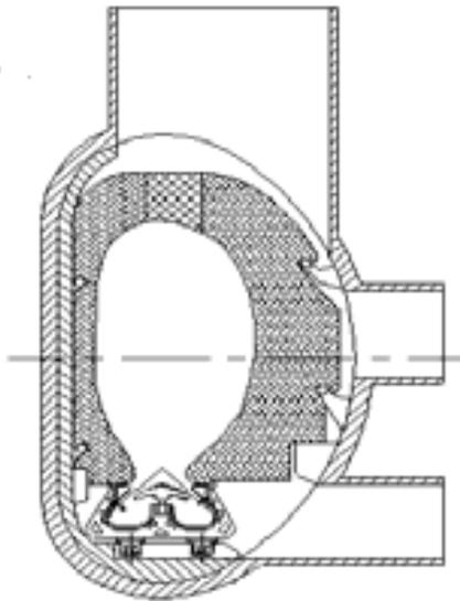
Attaching lock of blanket in vacuum vessel
