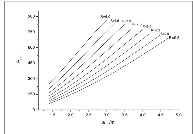
The current-drive power of a reactor with different sizes
