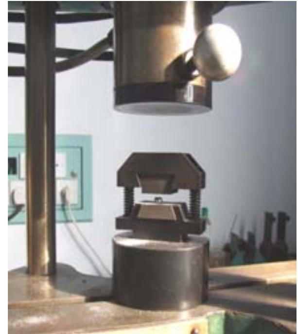
Press failure test device
